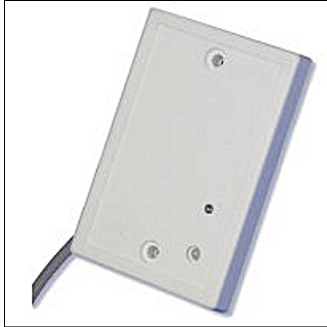
Figure 18 – The RFID Reader Used In Our Project, It's Mounted On The x/y Traverse.
