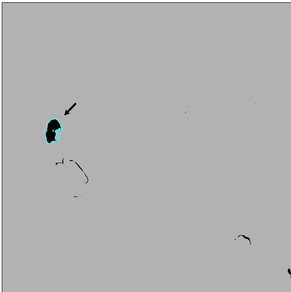
Figure 28 – Showing Particle Analysis With Parameter Adjustments: Only the Mussel Is Detected.
