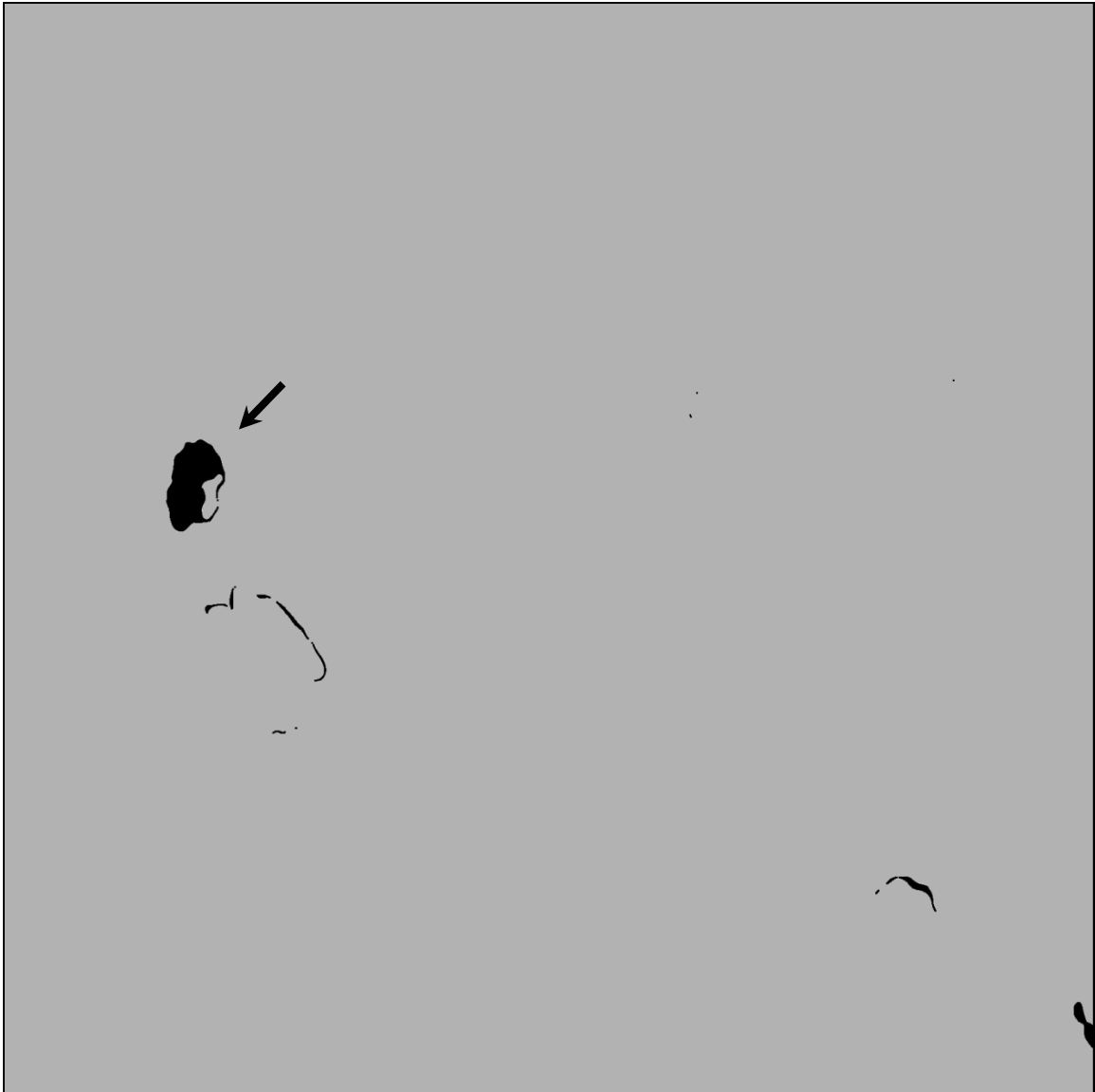
Figure 27 – White Shell Mask After Applying Dilate And Fill Holes Function With Arrow Pointing At The Detected White Shell.
